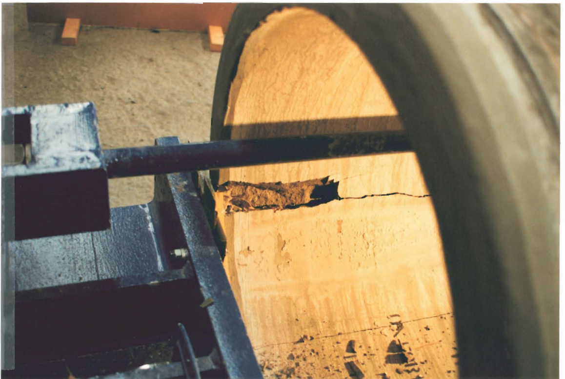
Plate D5 Pipe 6: Standard pipe ( 1.0^\circ deflection)
