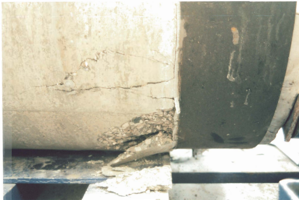
Plate D13 Pipe 3: Pipe with joint reinforcement (0.5° deflection)
