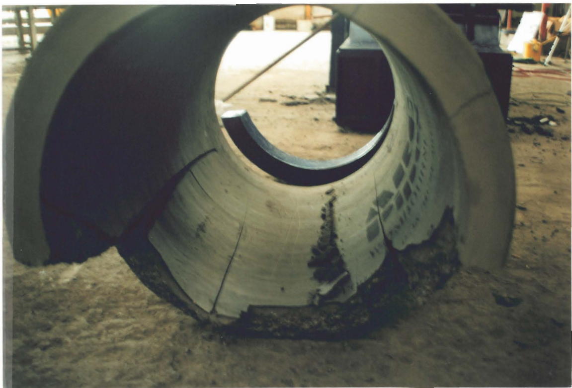
Plate D1 Pipe 2: Standard production with 3° chamfer (0.5° deflection)
