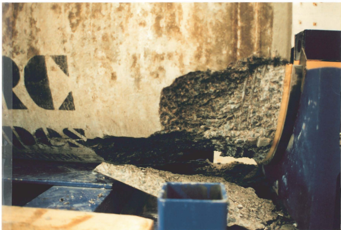
Plate D4 Pipe 5: Standard pipe with 3° chamfer and joint reinf't (0.5° deflection)
