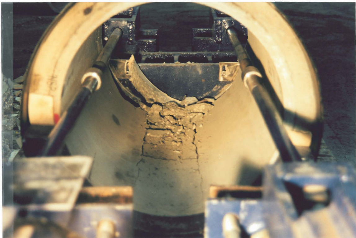
Plate D24 Pipe 14: Standard pipe unreinforced with 2° chamfer (1.0° deflection)
