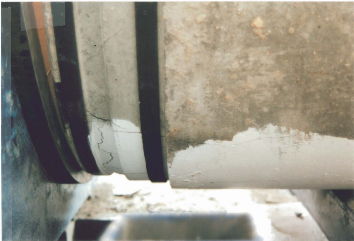
Plate D35 Pipe 11: Standard pipe with 1 presressed steel band (1.0° deflection)
