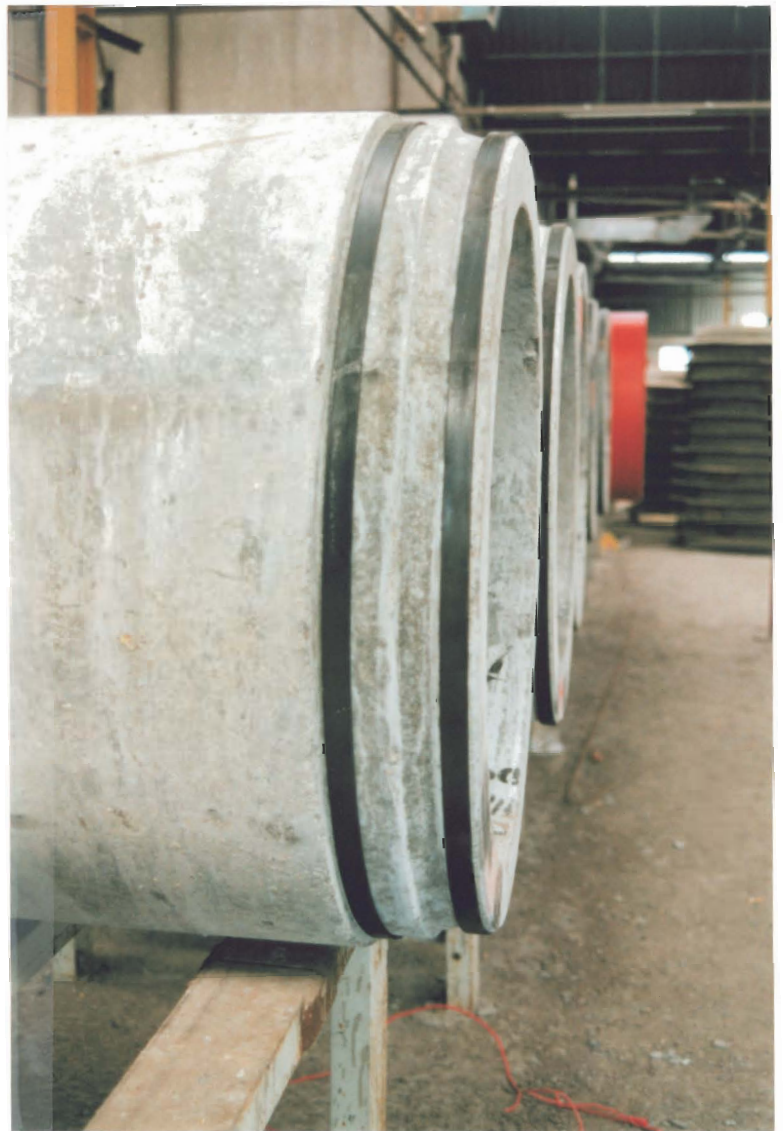
Plate 4.2 Modifications incorporated at the spigot joint of Hepworth pipes.
