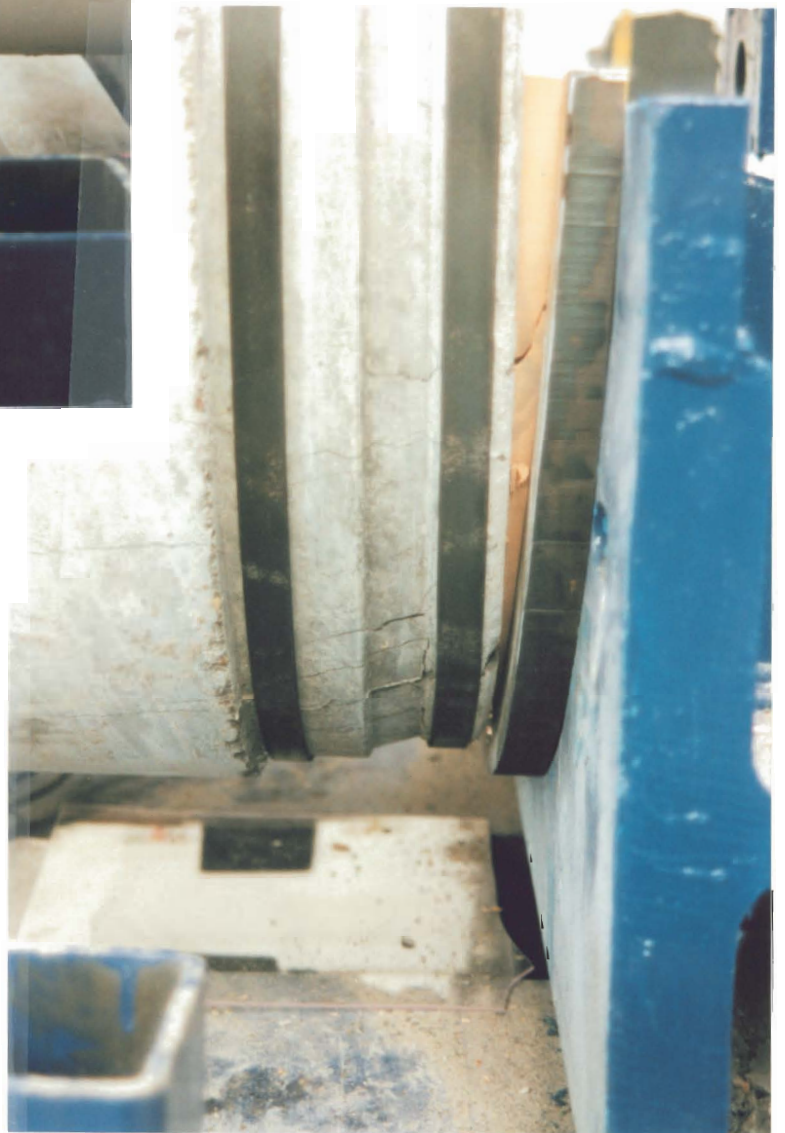
Plate D36 Pipe 12: Standard pipe with 2 pressed steel bands (1.0° deflection)
