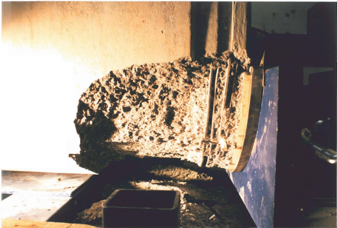
Plate D3 Pipe 4: Standard pipe with 3° and joint reinforced chamfer (0.5° deflection)
