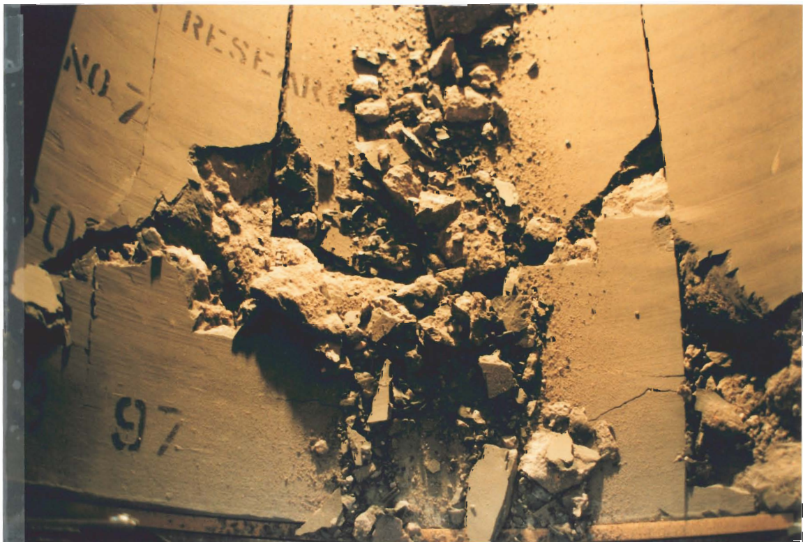
Plate D7 Pipe 9: Standard pipe with joint reinforcement ( 1.0^\circ deflection)
