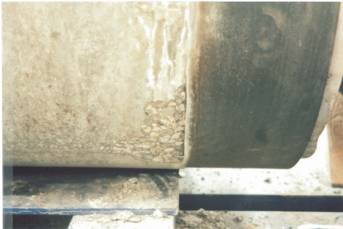
Plate D15 Pipe 5: Standard pipe with 3° chamfer and joint reinft (0.5° deflection)
