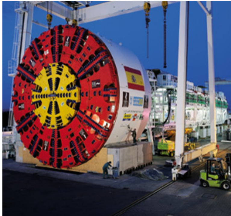
Figure 1.1. Herrenknecht S-300 Earth Pressure Balance Shield for Madrid. Maximum excavation diameter of 15.20 m and installed torque of 125268 kNm (Herrenknecht, 2006).
