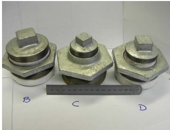
Figure 6.32. Gate discharge connectors and plugs; Diameters B = 71.5 mm, C = 45 mm, D = 51.5 mm.
