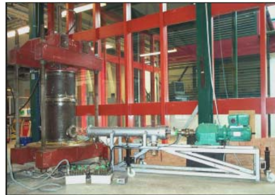
Figure 2.36. Overview of model EPB machine screw conveyor system at Cambridge University (Merritt, 2004)
